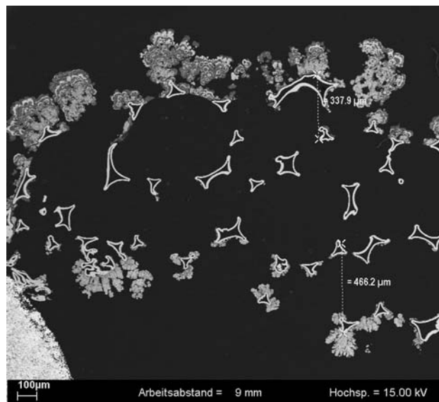
Fig. 3 Cross-section of Co–Mn–B deposit on RCM-Ni-4753.016 foam
